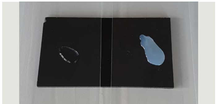
Figure 4: Water drop resistance testing of oil-modified dispersion (left) and standard ASR-based binder (right). The picture was taken after one hour of water drop exposure following 24 hours of drying at ambient temperature on glass.
