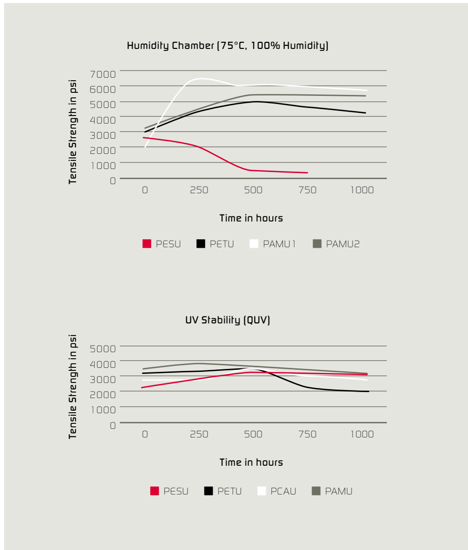
Figure 1: Hydrolytic stability (top) and UV resistance (bottom) evaluated in terms of strength retention.
