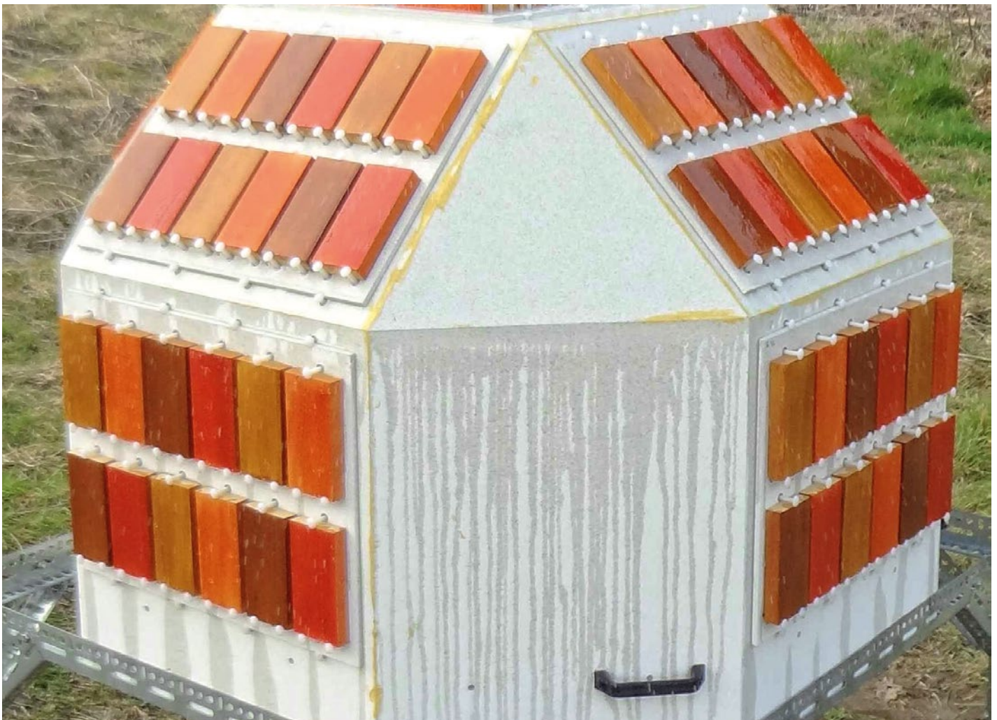
Figure 7: Novel multifaceted exposure rig (MFER). The same coating systems are exposed at four compass directions and with three inclination angles. Source: PRA
