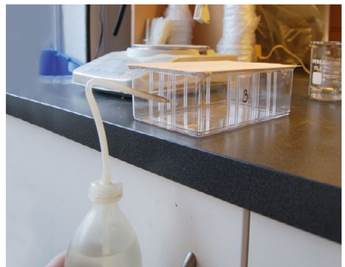
Figure 7: Filling with saturated salt solution through a 3 mm hole drilled in the side of cup.
