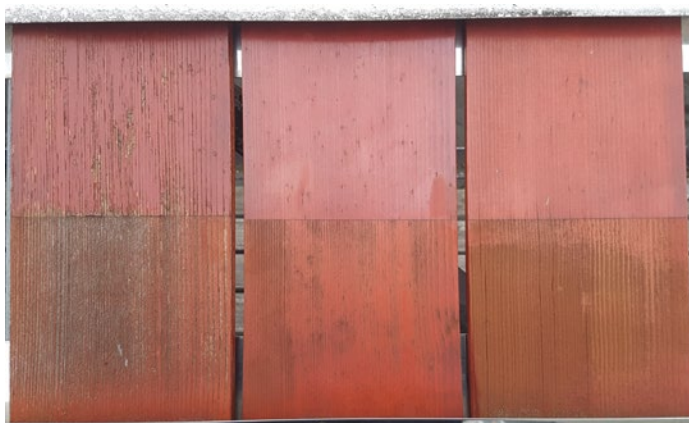
Figure 6: Outdoor testing results (Graz/Austria; 24 months; 45° south). From left to right: acrylic binder; oil-modified multi-domain dispersion; alkyd binder. Top of each board double-coated; bottom of each board single-coated.
